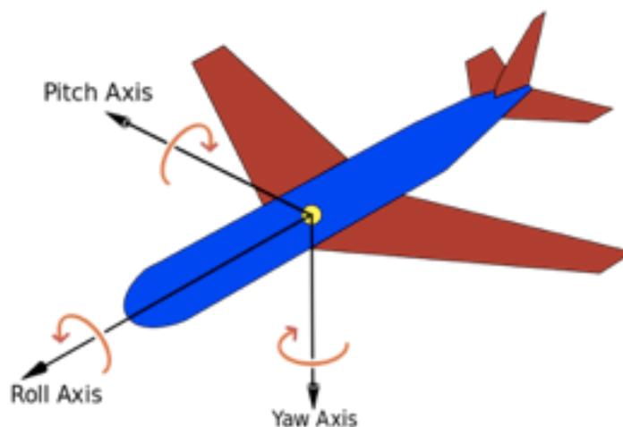
Figure 12 Pitch, Yaw and Roll on a Fixed Wing Aircraft
