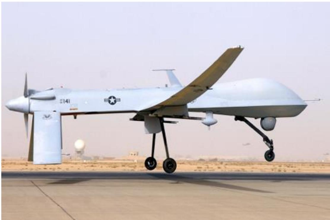
Figure 4 An MQ-1 Predator Unmanned Fixed Wing Drone prepares for takeoff
