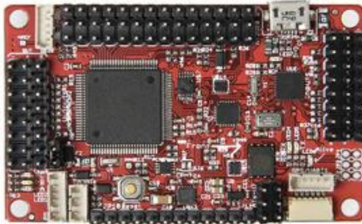
Figure 11 APM Flight Control Board (geetech.com)
