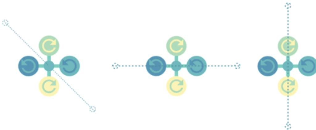
Figure 13 Yaw, Pitch and Roll Axes on a Quadcopter
