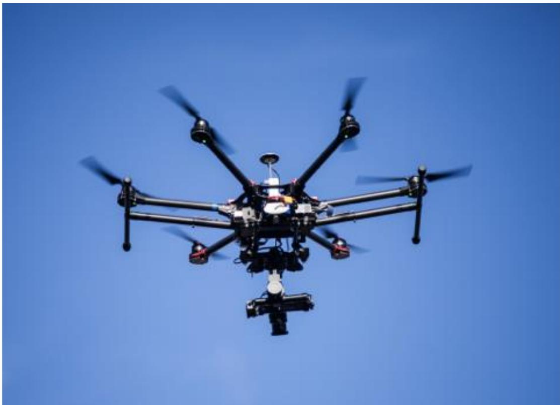
Figure 3 A Multi-rotor drone featuring six propellers
