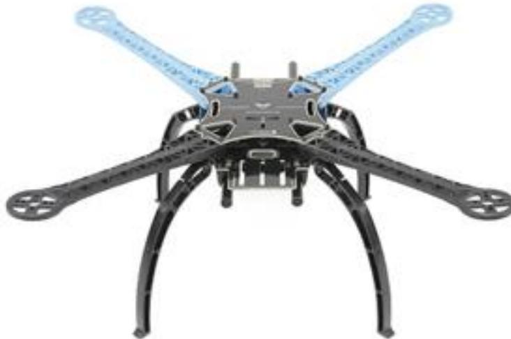
Figure 8 Quadcopter Chassis (hobbyking.com)
